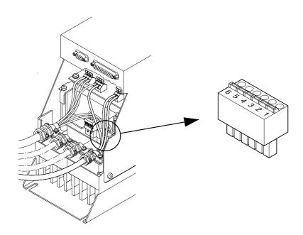
Plug type: 6-pole pluggable spring terminal (max. 1.5 mm<sup>2</sup> / AWG 16); from Phoenix, Mini-Combicon grid 3.81 mm
