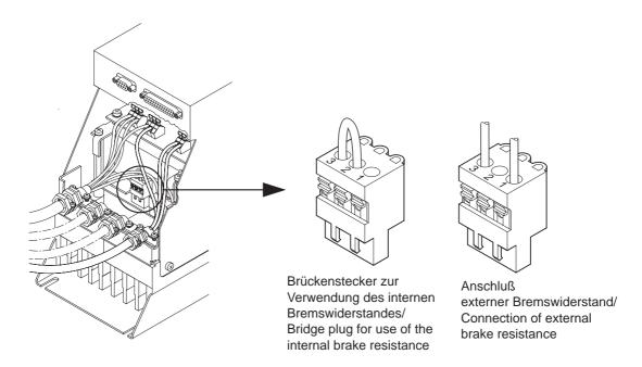
Plug type: 3-pole pluggable spring terminal (max. 1.5 mm² / AWG 14); from Phoenix, Combicon grid 5.08 mm
