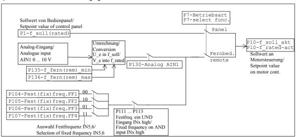
If parameter P7-select func. is set to Panel, the speed setpoint value of P1-f-rated is used, and the analogue setpoint value at AIN1 and the fixed frequencies have no function.
