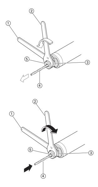
Insert replacement tool in the chuck. Turn nut (5) with spanner/wrench in direction of the arrow > tightening snugly, thereby securing the tool.
